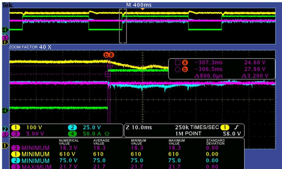
3. The sink mode can effectively absorb the reverse electromotive force and provide a safety test guarantee;
